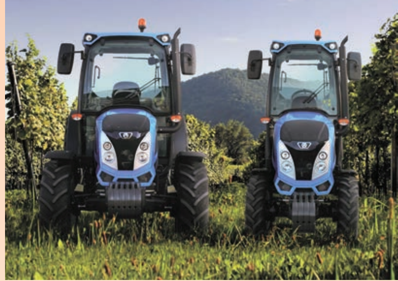
The new Rex 4 Series vineyard models can be as little as 1m wide, even the 111hp version.
