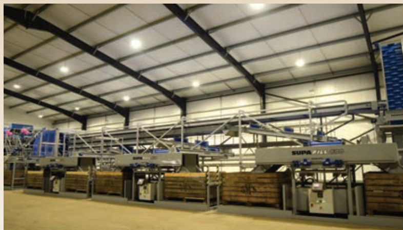
3Ms' new Haith SUPAFILL 600 grading line.
