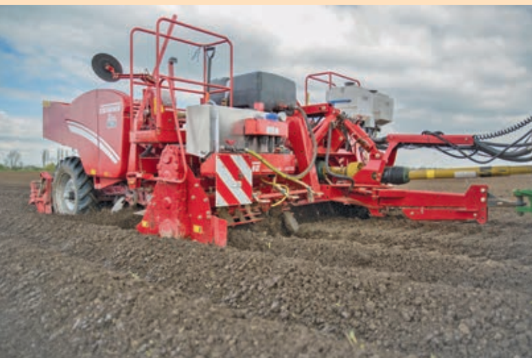
One of the farm's Grimme GL430T trailed 4-row potato planters in action.
